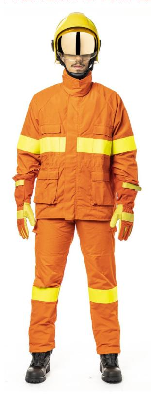
Complete composed of Jacket and Overall in meta-aramid Rip Stop IOR (hydro repellent oil) fabric with the composition 93% meta-aramid 5% para-aramid 2% antistatic fiber of 185 g/mq ca. **Oeko-tex®**.
