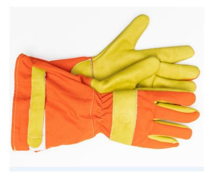
5 Fingers gloves with the palm in grain leather water-repellent to liquids. Back and cuff (cm18) in meta-aramid fabric lined with quilted meta-aramid fabric, reinforcement on the back at the knuckles in grain leather. On the bottom part of the palm reinforcement for vein protection in grain leather, elasticated back. Seams made of Kevlar® yarn. Sleeve adjustment by fastener with Velcro® tape. The gloves are equipped with a belt attachment system.
