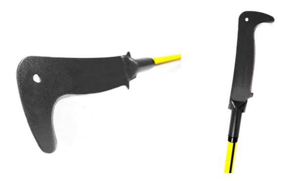
The **Tajamata billhook** is a tool implemented for aerial cleaning in firebreak lines and defense extension by eliminating fuel's vertical continuity. The sickle-shaped blade has a curved edge that allows cutting by sliding and its reach makes it ideal for small branches and bushes in mediumheight vegetation, since its head is especially balanced to optimize its effectiveness by decreasing accident risk due to involuntary deviations in the use resulting in a balanced product.
