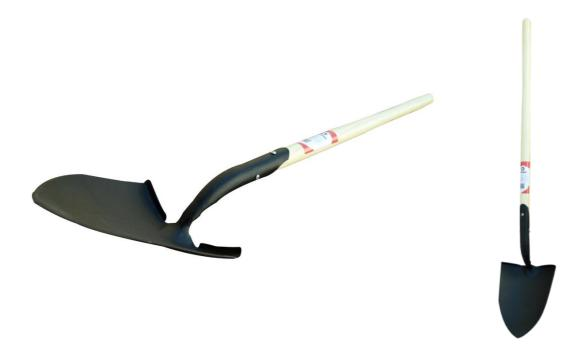
It is the main tool used for opening and extending lines of defense, excavating, and removing vegetation. It allows to clear up to mineral soil stopping fuel supply and the spread of fire. It is also widely used for prescribed burns, burnouts, control of secondary seats of fire, and mopping up operations.
