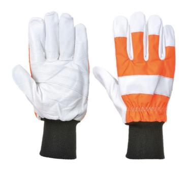
Anti-cut glove in full-grain leather, polyester and elastic. Designed to offer maximum protection and comfort whilst performing chainsaw tasks. Protective material in the left glove only to EN381-7 Class 0, 16m/s.
