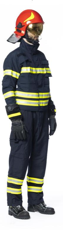
Forest firefighting and USAR suit model **TRENTO** in 185 g/m<sup>2</sup> meta-aramid fabric doubled on the front  $185+185 = 370 \text{ g/m}^2$ . It is flame retardant, antistatic, IOR (hydro oil repellent) Rip-stop (tearproof).
