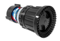
Nozzle with flow rates from 400-2000 l/min. The nozzle can be adjusted with a standard operating pressure of 7 bar, or in low pressure mode at 4 bar, by turning a knob located on the front of the nozzle. The flow of the water can be regulated by rotating the head to obtain a full jet or a spray jet up to 120°C.
