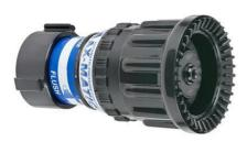
Automatic pressure control nozzle with a flow rate of 400/2000 l/min. The nozzle has its best performance at a standard pressure of 7 bar. The flow of the water can be regulated by rotating the head to obtain a full jet or a spray jet up to 120°C.
