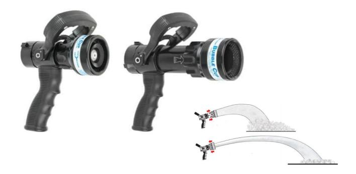
A unique combination nozzle capable of producing aspirated finished foam, conventional straight stream and a wide fog pattern. To use the **integrated aspirating foam-adapter** of the nozzle, the operator slides the outer sleeve forward: in this way the lance will create a "Venturi effect" and generate excellent foam. If an immediate wide fog pattern is needed, the sleeve can be retracted and adjusted instantly to its regular position.
