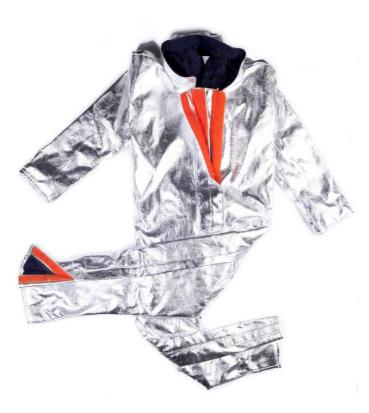
Fire Proximity **Overall ST710** composed by aluminized fabric SAFAL GREEN of 340 gr. (50% para-aramid 50% Panox), internally insulated with OXISTOP fabric of 325 gr which in turn has the following composition: felt in pre-oxidized fiber of 200 gr. quilted with lining in fabric 50% aramid 50% viscose FR of 125 gr.
