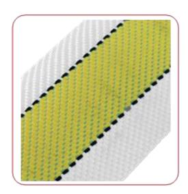
**Fire-fighting Hose High Pressure**: external circular weave layer of high tenacity polyester thread; elastometric waterproofing; special textile to maintain high performance. For special needs where higher pressure is required, JET H.P. hose is the best solution, with operating pressures **up to 40 bar**.
