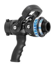
Nozzle model VORTEX SVFG made of anodized aluminium with ball valve regulated by a plastic handle. With 1.5" F swivel connection, threaded head for coupling nozzles of various diameters of: 12, 16, 19, 22, 24, 25, 27, 28, 30, 32 mm.
