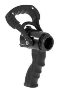
Model FP100 lance made of anodized aluminium with ball valve regulated by a plastic handle. With 1.5" F swivel connection, threaded head for coupling nozzles of various diameters of: 16, 22, 24, 25, 28, 30 mm.
