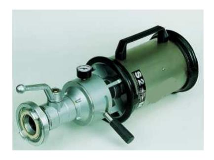
Made of aluminium and rubber in order to resist shocks and stresses. Low and medium expansion foam delivery, selectable by lever, foam expansion ratio: 1:4/1:10; ideal for the use of mixers of the "Z" line. Ergonomic handle, gradually opening flow opening lever, equipped with pressure gauge to control the inlet pressure.
