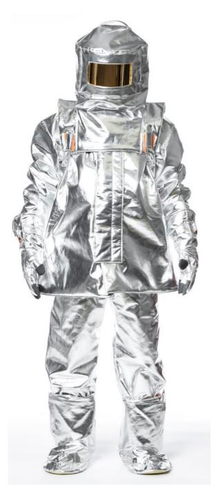
5-piece suit made with the new 520 g / m2 100% aramidic FCL aluminized fabric, and internally insulated in 485 g / m2 OIXISTOP consisting of 3 layers of 120 g 100% pre-oxidised felt, and a 125 g lining / m2 composed of 50% aramid fiber and 50% viscose FR.
