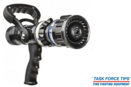
G-Force selectable nozzle with 5 flow settings:100-200-300-400-500 LPM, oerating pressure 6 bar.
