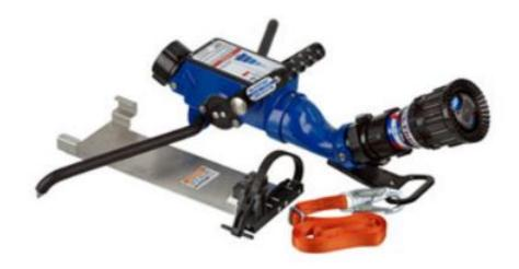
The BILTZ FIRE monitor has a flow rate of **400 liters up to 2000 liters per minute** with a maximum range of 61 meters. The monitor is designed to reduce the input and output frictions to a minimum, thus eliminating all the pressure drops.
