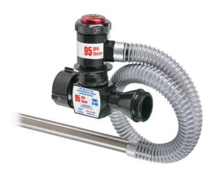
Equipped with 1.5" Female x 1.5" Male connections, complete with sunction tube and rotating mixing selector with positions of: closing (OFF) and mixing at 0,25% - 0,5% - 1% - 3% - 6%.
