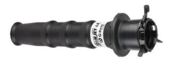
**TFT cod. FJ-LX-G** Air-aspirating low expansion foam-making attachment for all G-Force Nozzles medium pressure PN16. Provides excellent low expansion foam with a tight bubble structure. Is constructed of durable UV stabilized polyethylene, stainless and aluminium.
