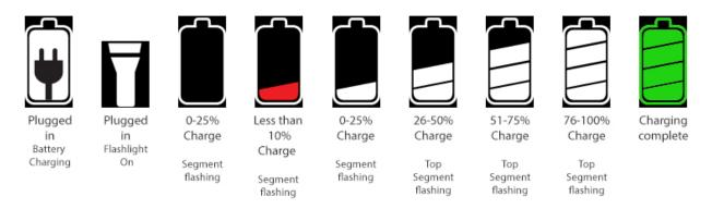
*NOTE:* Reveal FirePRO will provide up to 4 hours of imaging time with a full charge.
