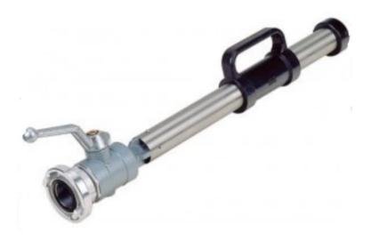
Low expansion foam nozzle. Stainless steel body complete with soft rubber handle. 2 "male threaded connection. With aluminum shut-off valve. Capacity 200/400 LPM. Compliant to EN 16712-3 Supplied with UNI and on request with STORZ, DSP, BSS connections.
