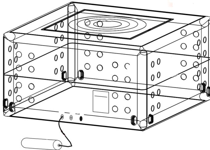
The supporting frame is equipped with overpressure valves which release a quantity of air at the moment of impact, which allows a body to be cushioned by absorbing its weight without making it bounce.
