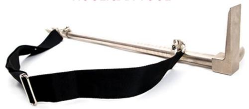
It is a multi-purpose bar used to penetrate, twist, cut, force or hit. It consists of sharpened claws or a recessed nail puller, a duckbill (chock or adze) and a conical pike, which is especially useful for quickly opening many types of doors. Nowadays **Hooligan hand tool** has become one of the most versatile hand tools used in the last six decades for a number of tasks in the field of fires. It is a tool that has a long tradition among structural fire firefighters.
