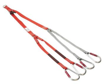
Lifting and transport bridles for Basket Stretchers. One central Snap link to be connected to the Helicopter Rescue Hook, with two adjustable belts and four belts with Snap Links. Made of resistant woven Nylon, supplied with Security Steel Snap Links.
