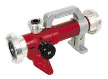
Particularly light and compact **foam mixer** indispensable for the correct mixing of the foaming liquid; equipped with a 2.5 mt. suction tube with a rigid steel terminal for suction from a STORZ 25 connected thread.
