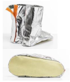
Over-boots composed of aluminized fabric SAFAL GREEN 340 gr. and completely insulated with quilted fabric OXISTOP 325 gr. with the lining 50% aramid 50% viscose F.R 125 gr. 100% meta aramid Sole reinforced with 100% viscose F.R fabric and closure on the back with Velcro® F.R. Sewing stitch in Kevlar®.
