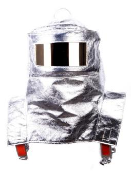
Integral lined Hood in aluminized fabric SAFAL GREEN of 340 gr. (50% para-aramid 50%Panox), completely insulated with fabric OXISTOP of 325 gr. Composed of: felt in pre-oxidized fiber of 200 gr. Quilted with lining in fabric 50% aramid 50% viscose FR of 125 gr.
