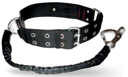
Waist belt with loops of support in accordance with **EN 358** and fitting with built-in carabiner 85 mm wide polyester belt, and on the parts adjustable with aluminum edges; holes and slots overlapped reinforced with steel hook; finals are oblique; with adjustable buckle latching double aluminum.
