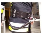
Belt positioning according to UNI EN 358: 2001 and according to DIN 14927
