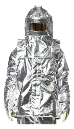
Jacket in aluminized SAFAL GREEN fabric of 340 gr (50% para-aramid 50% Panox), completely insulated with 100% pre-oxidized OXISTOP of 325 gr. composed by: felt in pre-oxidized fiber quilted with lining in fabric 50% aramid 50% viscose F.R.
