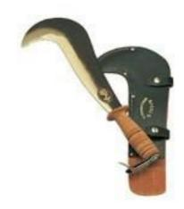
Billhook with short handle consisting of a series of non-slip leather discs, leather handguard, galvanized steel hook fixed at the end. Sharpened C55 HRC 55/58TAG forged steel blade, sharp, ready to use.
