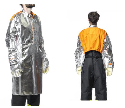
Unlined heat resistant apron composed on the front and sleeves by 340 g SAFAL GREEN aluminized fabric with the composition 50% para-aramid 50% Panox®.
